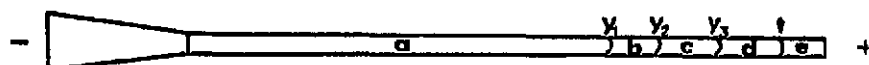
Fig. 1. Substances classed into five groups according to their mobilities in relation to the mobilities of the coloured reference substances Y 1 , Y 2 , Y 3 and indigotetrasulphonate (Table II). The area between Y 1 and the cathode was termed zone a; between Y 2 and Y 1 , zone b; between Y 3 and Y 2 , zone c; between indigotetrasulphonate (t) and Y 3 , zone d; and between t and the anode, zone e.
